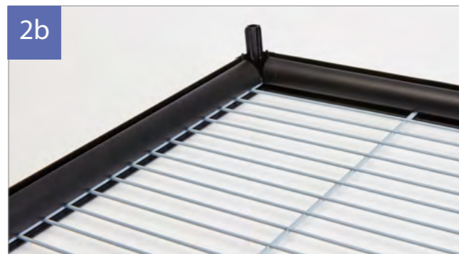
Slide the roof panel into the roof profiles. Make sure the thick vertical wires are facing downwards. Attach another top corner piece on the other side of the short roof profile.
