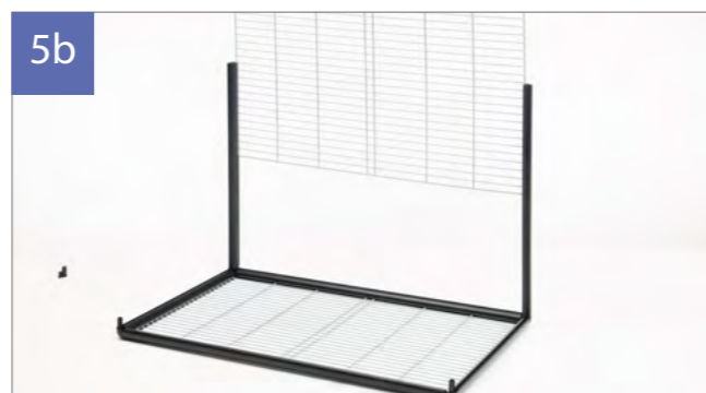
Attach 2 side profiles of 512 mm (f) on the roof. Slide the back panel (b) into those 2 profiles. Make sure that the vertical wires of the panel are facing outwards.
